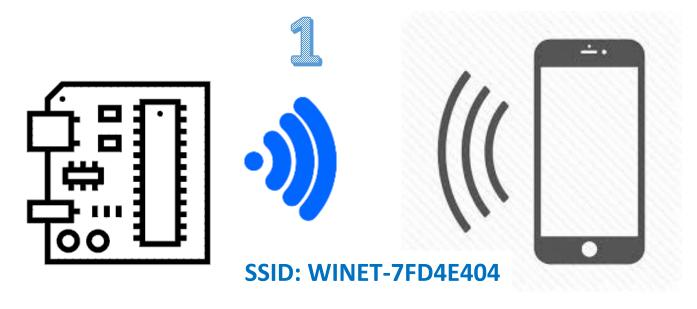
To setup the module, connect (with a smartphone, tablet or laptop) to the self generated network (SSID begins with WiNET followed by the last 8 digits of the MAC address). The WPA key is printed on the label outside the package.
