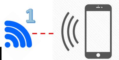
The first network is self-generated by the module and can be accessed using the WPA key (password) printed on the label of the device. It has to be used to setup the second WiFi connection.
